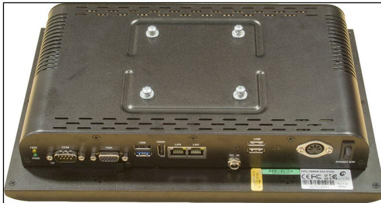
3. Remove the screws, washers and lock washers from the back of the ForneyLink and set aside.
