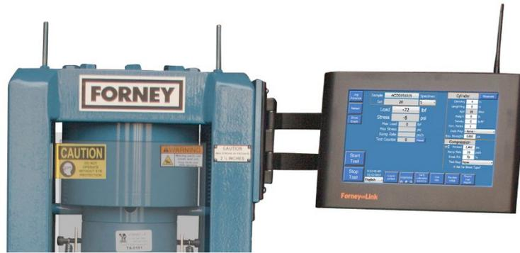
ForneyLink™ Touchscreen Interface is a powerful device which enables setup of testing protocol, real-time display of test data, and post-test data transfer.
