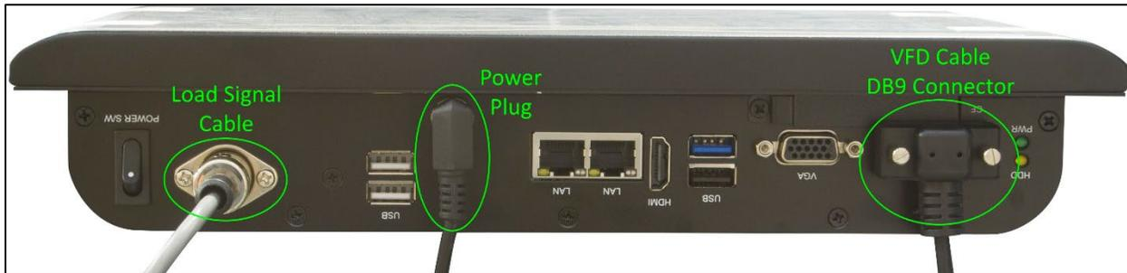
8. If your machine has additional USB connections for factory-installed options such as MOE, it is important to note that only the blue, USB 3.0 connector should be plugged into the blue USB 3.0 port on the ForneyLink. You can connect other connectors to any available USB ports on the ForneyLink, except for the blue, USB 3.0 port.
