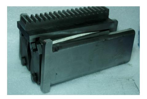
Finally place this assembly (one in the top and one in the bottom) into the machine and rotate the handle to grab the assembly and pull it up into position:
