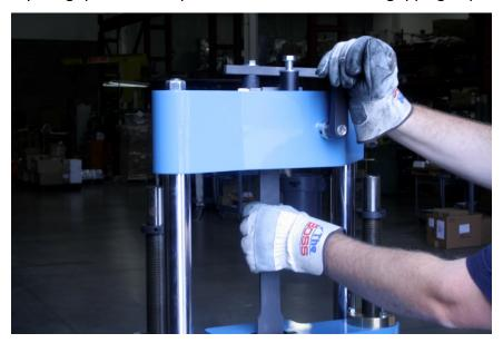
It is ok for the grips to protrude slightly out of the top (towards the grip keeper guard) while gripping. The grip should never come out of the bottom of the upper crosshead during gripping or testing! Check the grip model and specimen size if this occurs. These rules apply oppositely to the middle crosshead. The grip can come slightly out of the bottom but never the top of the middle crosshead.
