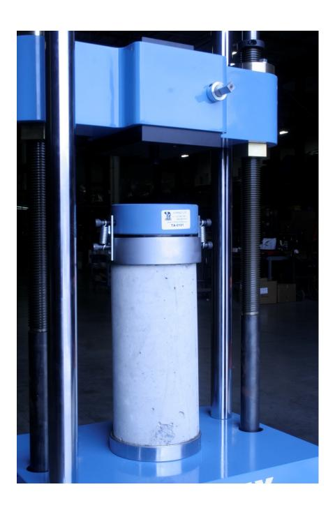
Tighten this bolt fully, so no daylight exists between the blue seat of the breaking head and lower black alignment plate. The finished assembly is shown the image below.
