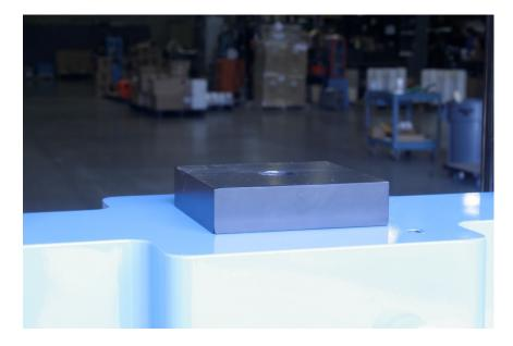
Next, install the bottom alignment plate on the bottom of the middle crosshead using the two mounting holes and socket head cap screws. These holes align with the same holes used for the grip keeper guards. Tighten the socket head cap screws with an Allen wrench.
