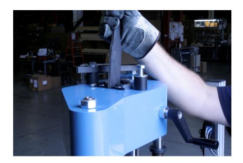
A proper grip is achieved when the grip contains approximately 3.5" length of tensile specimen filling the grip AND the grip is contained in the crosshead. Turn the handle to grip the specimen. Ideally the grips will be fully inside the crosshead while gripping a specimen.
