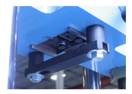
If any slippage occurs, sometimes it is necessary to hold the handle in the grip position on the middle crosshead and start the test until the teeth of the gripper set in the specimen. The handle should be removed after the teeth set and the test is underway.
