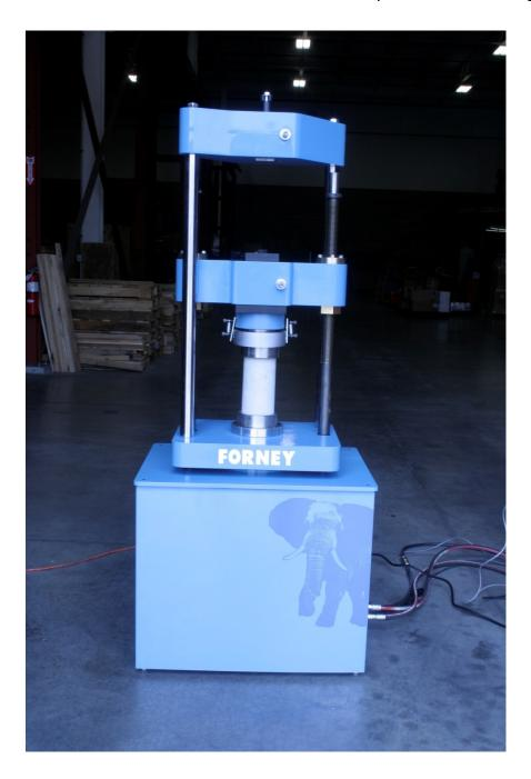
Start by removing any installed grips and the grip keeper guards from the middle crosshead.
