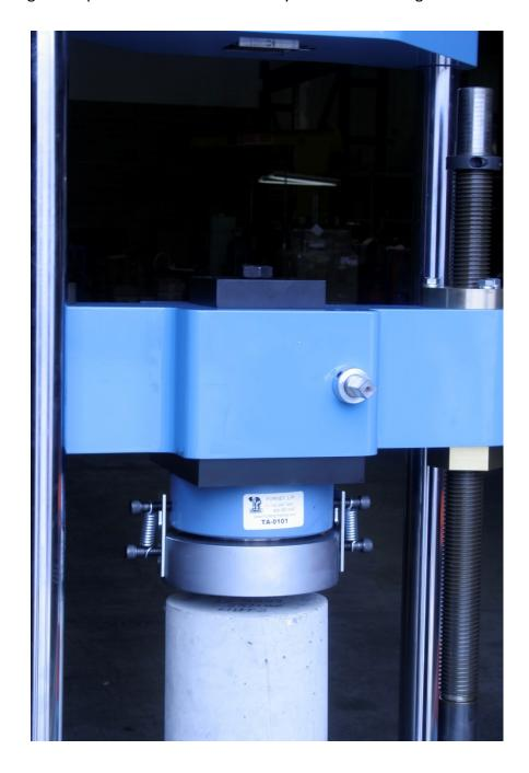
Finally, proceed with the compression testing portion in the CA-0399-LT-60 manual. Note many different compression breaking heads can easily be installed using this method.
