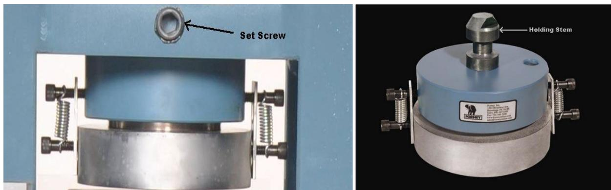
Figure 1 - Set Screw and Holding Stem locations
