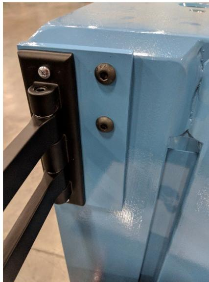
Once the mounting bracket is mounted to the frame, fasten the ForneyLink™ to the bracket with the included mounting screws.
