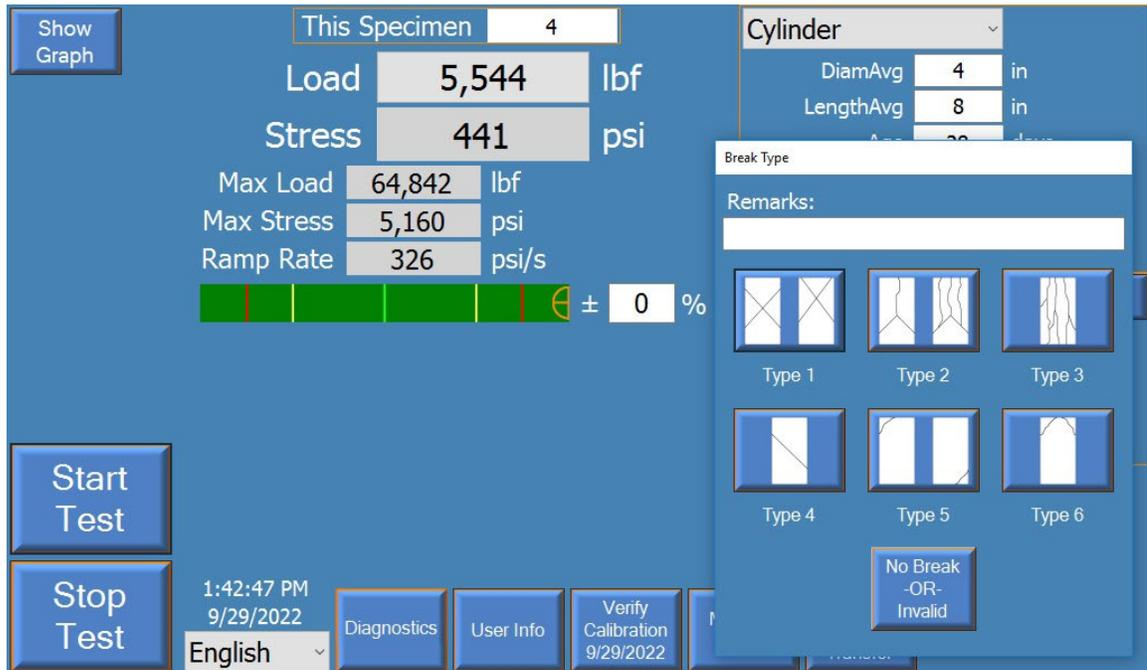
11. Record the Load at Break, or Stress at Break as desired, or simply move on to the next test if the data-logged results are used.
